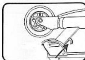
2. Pull the lever upwards.
