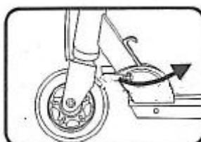
4. Lock the locking mechanism.
