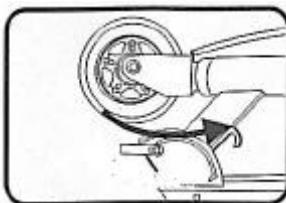
1. Unlock the locking mechanism.
