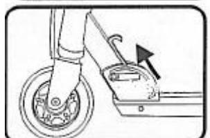
3. Pull the lever upwards.
