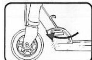
2. Open the locking mechanism.
