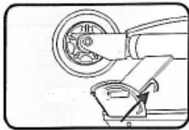
2. Pull the lever upwards.
