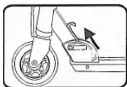
4. Pull the lever upwards.
