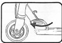
3. Open the locking mechanism
