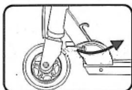
4. Lock the locking mechanism.
