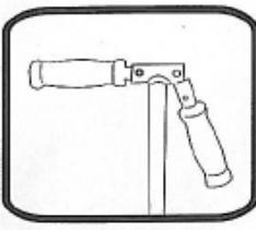
2. Remove both handles from the transverse steering wheel tube.
