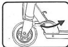
3. Lock the locking mechanism.
