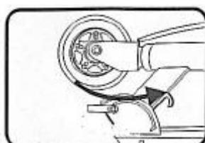
1. Unlock the locking mechanism.
