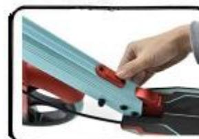
2. Press down on the folding mechanism and unfold the scooter.
