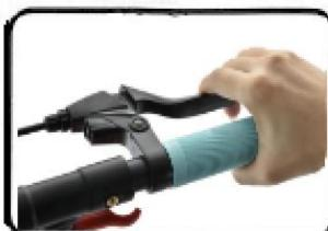
Hold the brake handle to check if it works properly.
