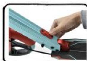
4. Press down on the folding mechanism and fold the scooter.
