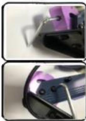
4. The folding part may be loose after long use. Use tools to adjust the screws under the folding part and tighten them securely. Make sure the folding system is in the correct position.
