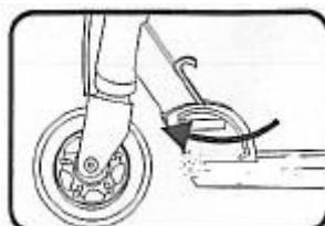
3. Open the locking mechanism.
