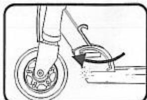
3. Open the locking mechanism.
